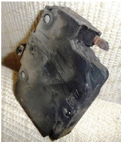
Fig. 5. 15 amp Stab-lok® Breaker (Note Smaller Connection Point)
