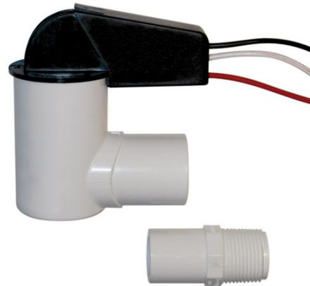
Adding a float switch to a plumbed auxiliary pan provides a high level of protection, but the 2006 IMC is good with the switch alone. In some cases, especially during replacement or upgrade work, installing the actual plumbing to handle the condensate flow from a secondary drain or auxiliary drain pan can be difficult. The use of float switches instead of piping is becoming popular.
