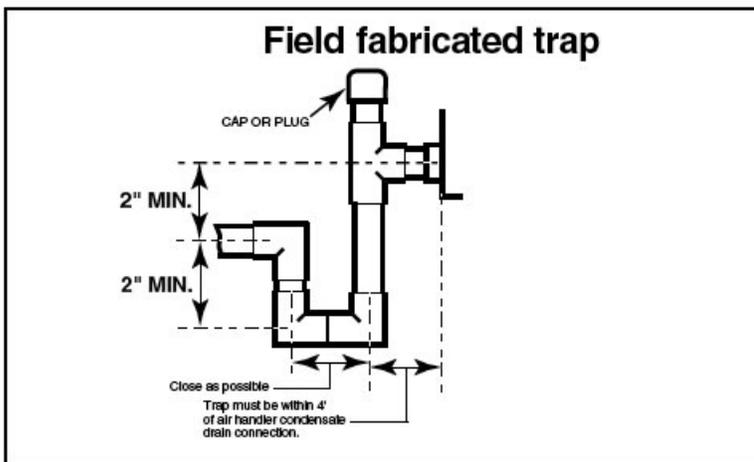
Recommended trap configurations. Illustration from Trane installation manual.
